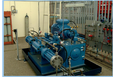
Forty horsepower single-stage unit for 12,000 psi discharge pressure.
